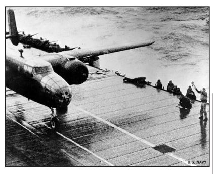
An Army Air Forces B-25B bomber awaits the takeoff signal on the flight deck of USS Hornet (CV-8), as the raid is launched, April 18, 1942. Note Flight Deck Officer holding launch flag at right, and white stripes painted on the flight deck to guide the pilot's alignment of his plane's nose and port side wheels.
